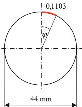
$$\frac{0,1103 \text{ mm}}{\pi \cdot 44 \text{ mm}} = \frac{\varphi}{360^\circ} \Rightarrow \varphi = 0,287^\circ$$
